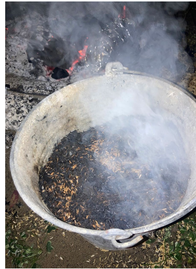
Burning the rice hulls in a bucket directly over the flame yielded the best results with minimum lost of RHA, and a reduced amount of foreign particles.
